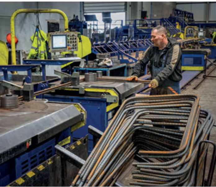
Armasteel's activities as a bending centre are entirely made to order, cutting and bending steel for large contractors' construction sites and delivering it directly to the job.
